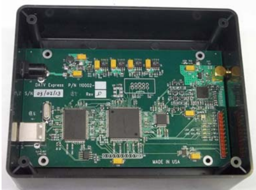
Fig 04 – the DATV-Express exciter board is a single printed circuit board.
