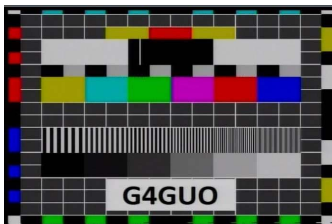
Fig 10 – Test pattern received using DVB-T protocol with 7 MHz bandwidth on 1.3 GHz
