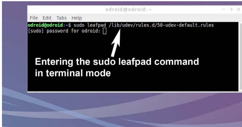
Figure 8 – TERMINAL mode command-line window while typing the “sudo leafpad” command
