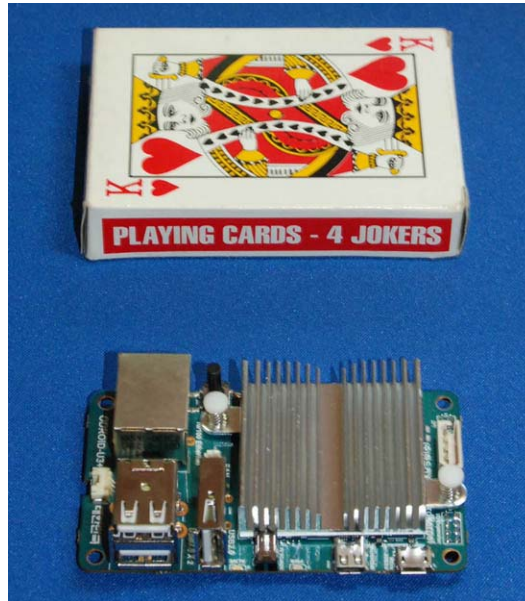
Figure 2 – Size of quadcore-ARM ODROID-U3 board is about the same size as Raspberry Pi
