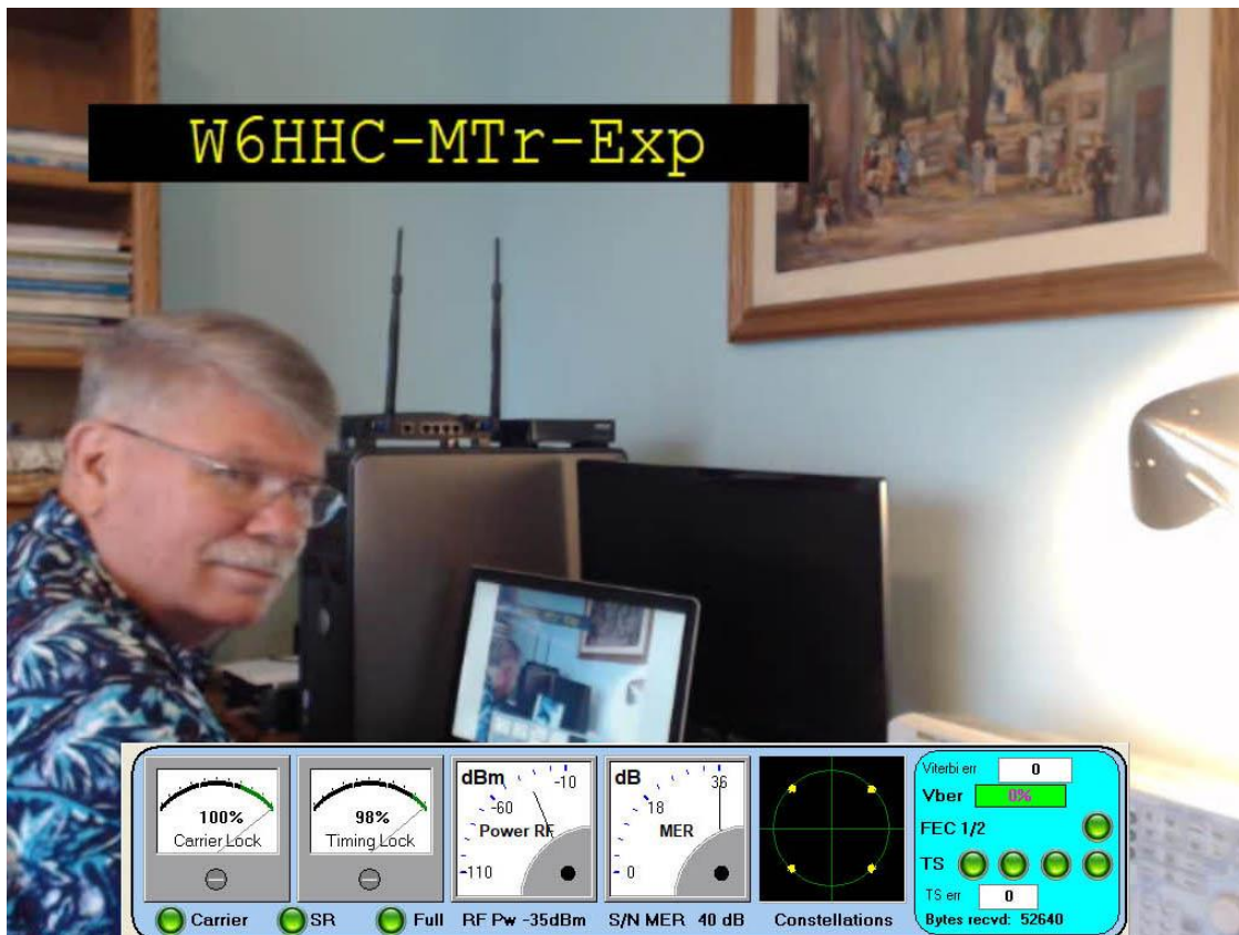
Fig 03 - The MiniTioune software is shown in receiver-mode for DVB-S. The Measurement-Panel at bottom can also be removed.
